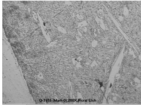
Fig. 1: Optical Microstructure for the Cross-section of SS304 Steel Hardfaced by Electrode 1
